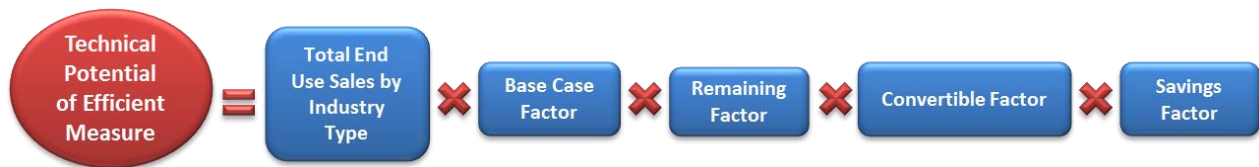
Equation 5-2: Core Equation for Commercial Sector Technical Potential
