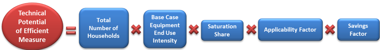
Equation 5-1: Core Equation for Residential Sector Technical Potential
